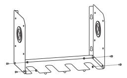
Attach the two side panels to the middle shelf using two bolts and nuts per side.
