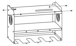
Position the support bar so the slot passes through the tab on the bottom shelf with the power tool slots. Secure the bar by lining up the hole at the top of the support bar with the corresponding hole on the middle shelf. The support bar should be positioned behind the front edge of the middle shelf. Secure using a bolt and nut.
